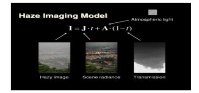
where J(x) is the scene radiance or haze-free pixel color, T(x) is the transmitivity along the cone of vision, and A is the atmospheric intensity, resulting from the environmental illumination.
