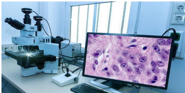
Figure 3.2: Device used to digitize histopathological image
